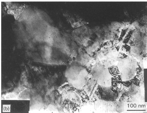
Figure 6 (a,b) TEM of nanocrystalline Ni performed 2 min after keeping a constant temperature of 623 K.
