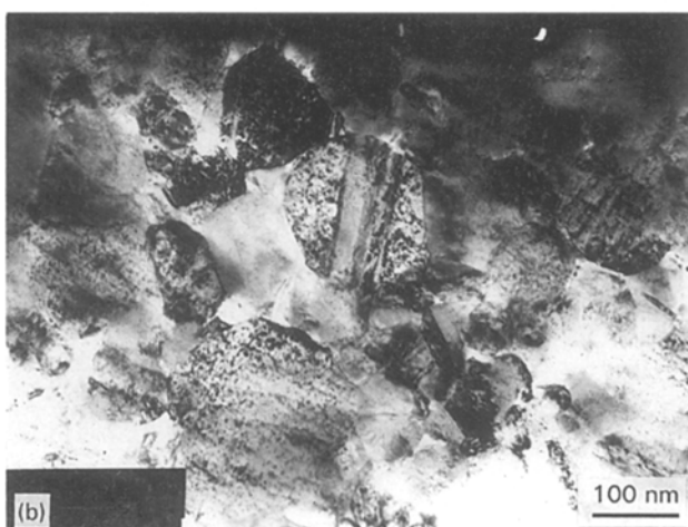
Figure 1 (a, b) TEM of the initial nanocrystalline Ni with mean grain size of 70 nm.
